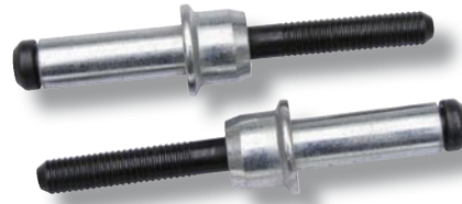
Avbolt® 3/8", 1/2" and 5/8" (10 mm, 12,7 mm and 16 mm): 3 piece design (sleeve, collar, stem)
